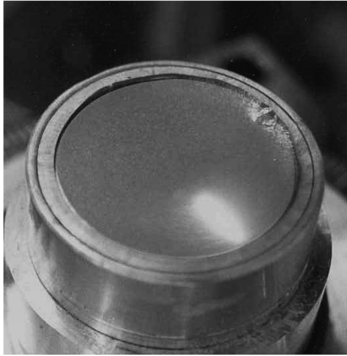
Figure 1.5 A long spark created by using a cylindrical lens, on a filter set on a rotating stage
