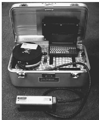
Figure 1.7 A portable LIBS surface analyzer, circa 1998
